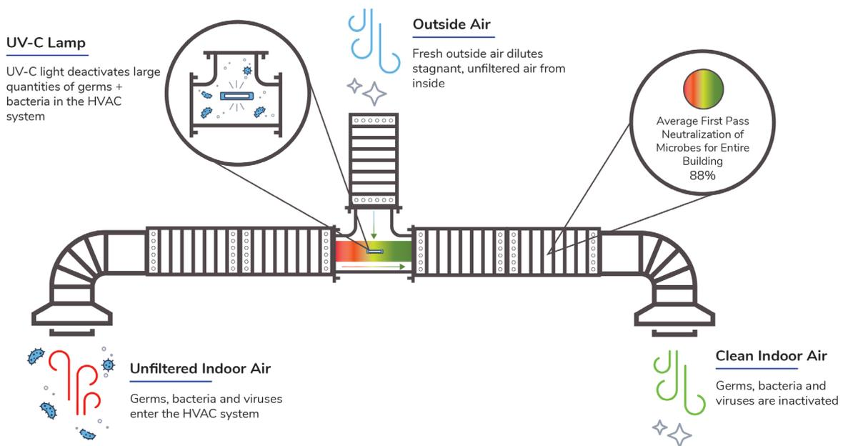
EMC confirmed the efficacy of the system using a proprietary mathematical model, specific to in-the-field HVAC performance, that predicts microbe neutralization. These calculations addressed: Duct size and air flow rate, UV-C lamp irradiance levels and microbial resistance to UV.
